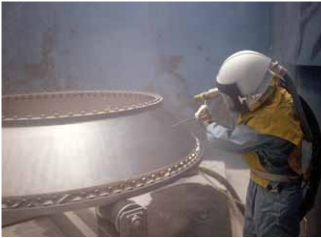
The glass beading process before the IES improvement project. Here, the technician is manually glass beading a section of the reusable solid rocket motor.
